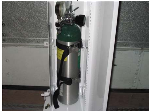
O2 Tank secured in the O2 Bus Buddy™
